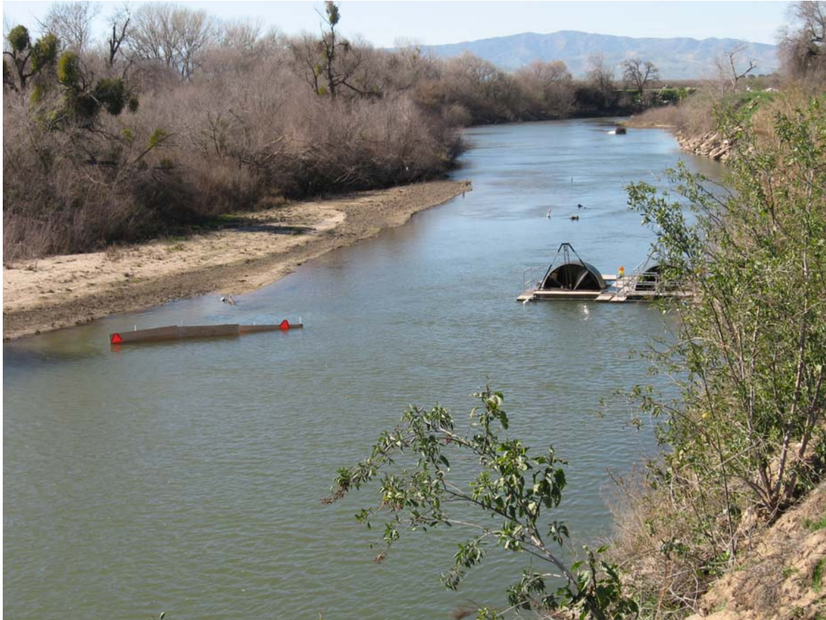
Figure 3. Grayson rotary screw traps with “weir” structure approximately 50 feet upstream of the traps on the opposite bank.
