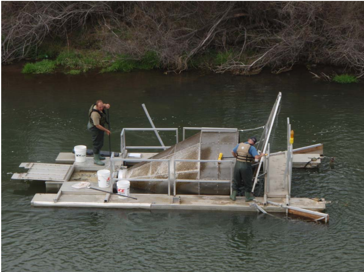
Figure 2. Waterford rotary screw trap with “wings” attached to the upstream end of the pontoons.
